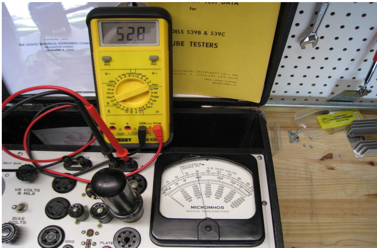
A 6L6 being tested with a 539B showing Gm & PLATE CURRENT.
