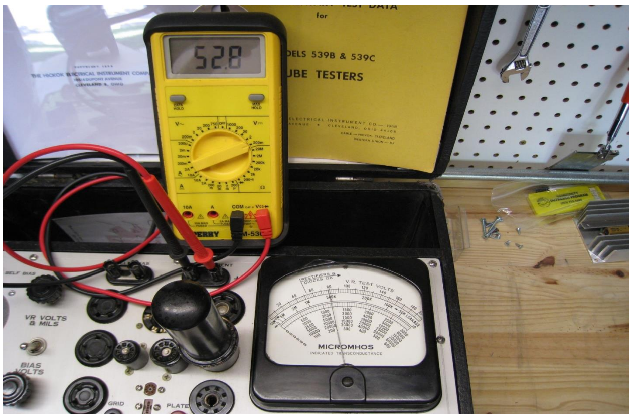
PICTURE SHOWS A 6L6 BEING TESTED FOR G m and PLATE CURRENT. Digital multimeter is set to read 200mV and is indicating 52.8 mA
